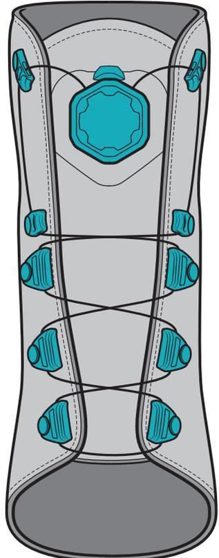
Top two 10mm paired guides should be located near the top of the collar of device.
