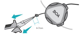
b) Determine lace length needed. Leave a maximum of 15cm of lace capacity per lace port.
