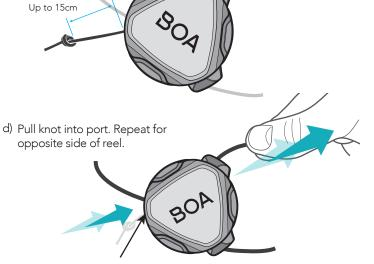
Note: Knot and tail should not be visible when the lace is seated properly.
