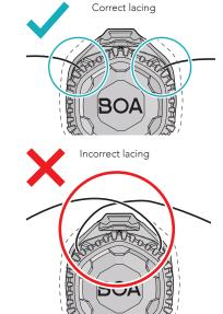
8 Hold lace lock with pliers. Push lace through back of hole, then loop lace around backside and through the second hole. Lace tail should be 2.5mm-5.0mm.
