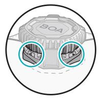
Fully insert flat-head screwdriver into one of the two ports. Use tool to pry reel upward untill cartridge pops out of bayonet.
