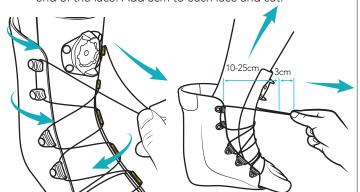
6 Press down on new reel to ensure it is closed. Turn the dial until the two arrows align.
