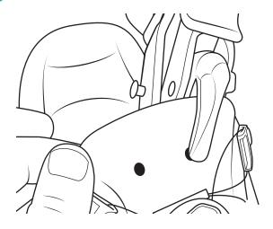
5 Snap rivets as described in step 2. If satisfied with placement, secure using QuickFit™ Tool.
