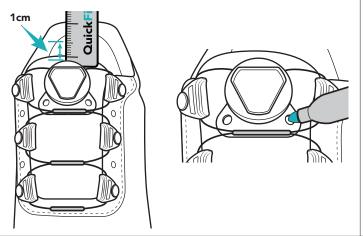
4 Punch holes using the 1/8" punch option of QuickFit™ Tool.
