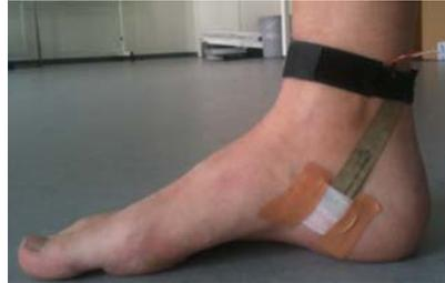
The strain sensor is thin, flexible and robust capacitive sensor allowing for in-shoe measurements
